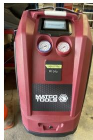
These vehicles use electric motors to run the AC compressor. The oil used to lubricate regular compressors conducts electricity, so special oils must be used. Special equipment is required to service them.
