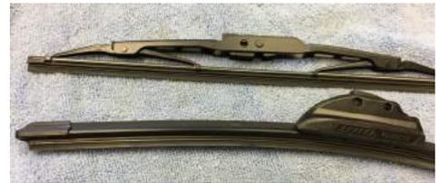
Below is the new design, called a “beam blade” with the metal reinforcement made into the rubber. Voila, no weird freezing shapes in freezing temps.
